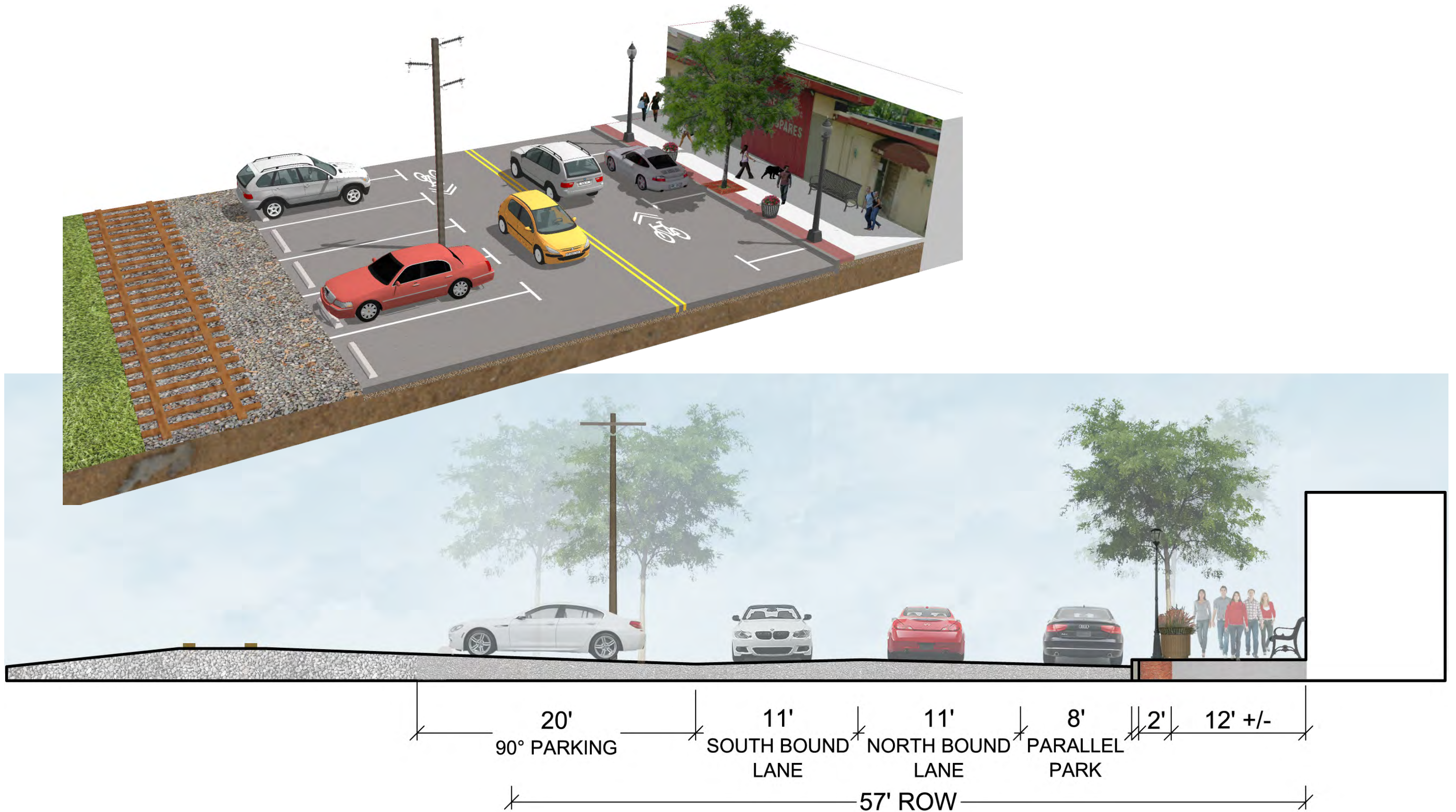
EXISTING BLUE ASH ROAD SECTION & ELEVATION
